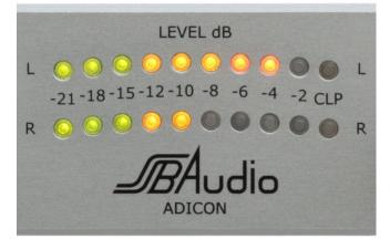
the analog signal. That is why there are no positive values on its scale, because the signal is either within limits or it is clipped, but a digital signal cannot exceed its range of numerical values. Clipping is indicated by the red LEDs **CLP**.
