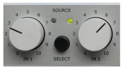
reduced to total silence. Instead, the gain of the input stage can only be set in a range from -10 dB to +20 dB.
