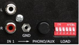
at high frequencies. The minimum load capacitance of the ADICON is 100 pF.
